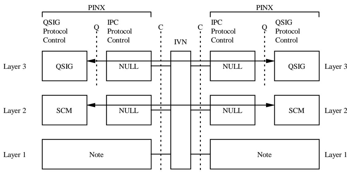
**Figure 6.3 — Protocol Relationship between Q/C Reference Point**
