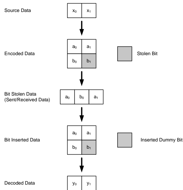
Figure 18- An example of bit-stealing and bit-insertion for R=2/3 code
