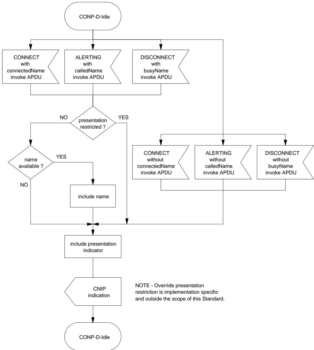
Figure B.4 - SDL Representation of SS-CONP at the Originating PINX
