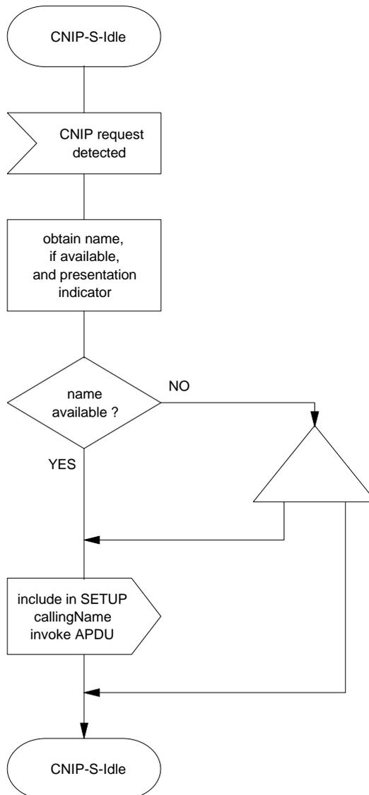
**Figure B.1 - SDL Representation of SS-CNIP at the Originating PINX**
