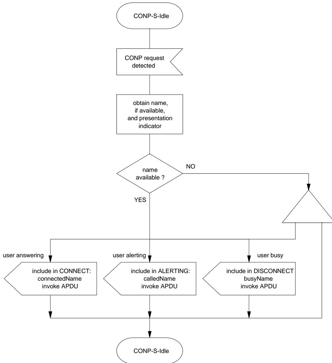
Figure B.3 - SDL Representation of SS-CONP at the Terminating PINX
